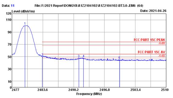
Dis. / Ant. : 3m 2020 MCTD1209-3006 Ant. pol. : HORIZONTAL Limit : FCC PART 15C PEAK Pressure : 101.7kPa Env. / Ins. : 23.2\*C/52.5% Engineer : Lynn
