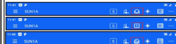
④ Select the prism, and slide to open [Menu] → [Prism Constant] to set the prism constant. Slide to open [Menu] → [PPM] set temperature, air pressure, and correction coefficient (as shown on the left).
