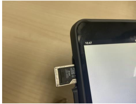
Figure 1-4-7 Installation of Micro SD card
