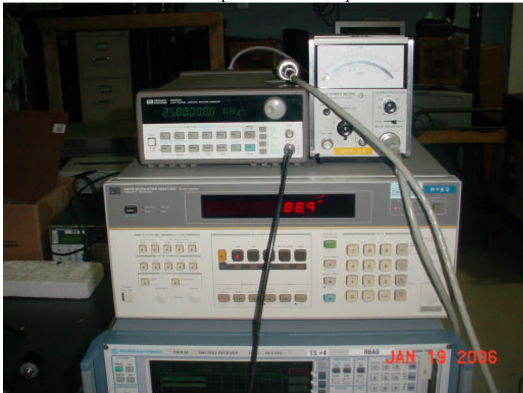
Test Setup for Modulation Characteristics
