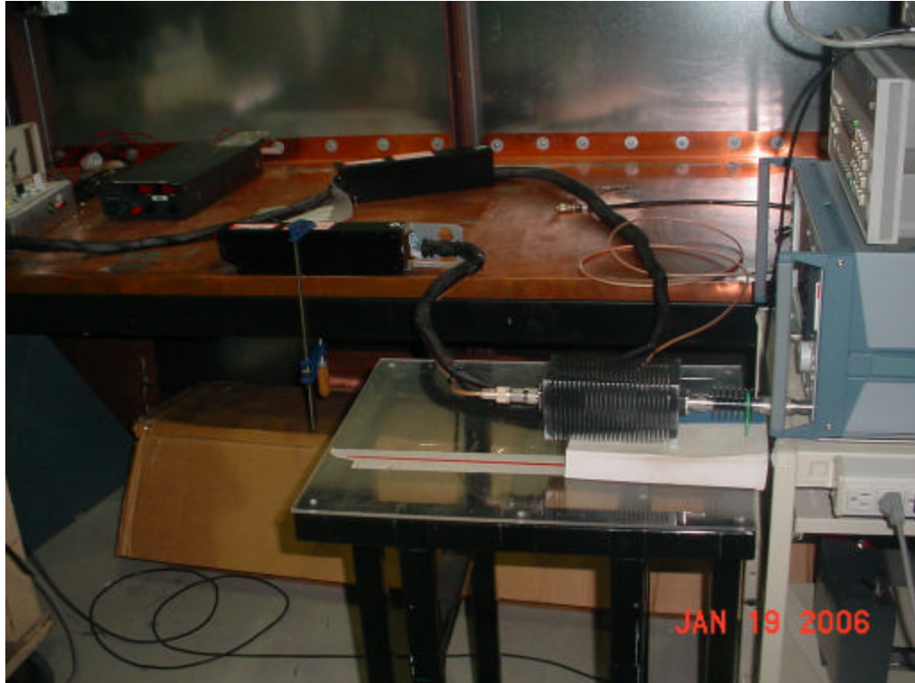
Test Setup for Occupied Bandwidth, Emissions Limitations, and Spurious Emissions at Antenna Terminal
