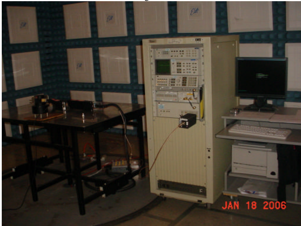
Test Setup for Antenna Conducted Emissions Tests, Receive Mode – 30MHz to 2 GHz
