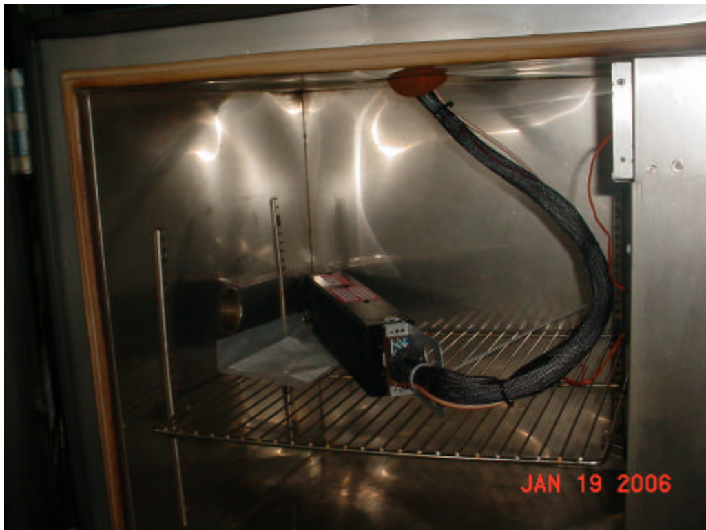
Test Setup for Frequency Stability
