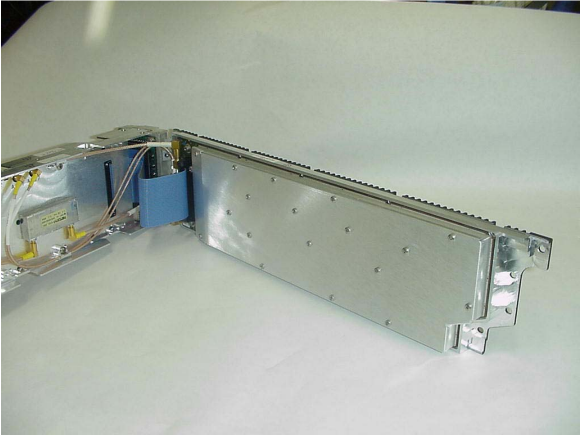
Photo 8: View of RF Circuit Card in shielded assembly.
