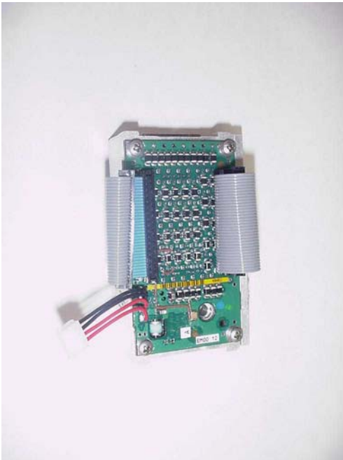
Photo 5: Rear Interconnect Circuit Card, Top View
