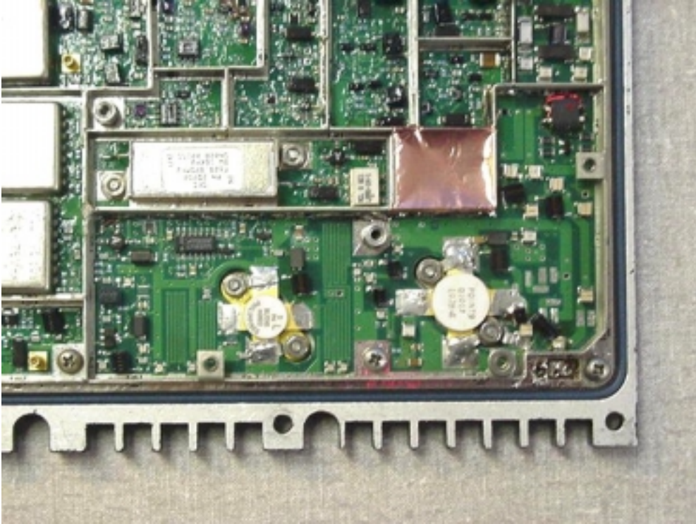
RF CCA, A1, Area around Power Amplifier
