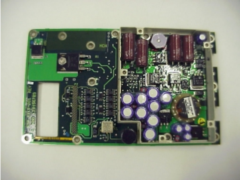
VDL Power Supply, A4, seen from the top side, shields off.
