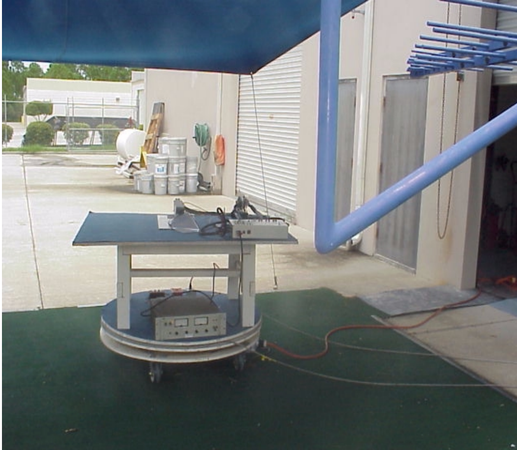
Test fixture at Rubicom (Testing Contractor) showing setup for radiated emissions testing.
