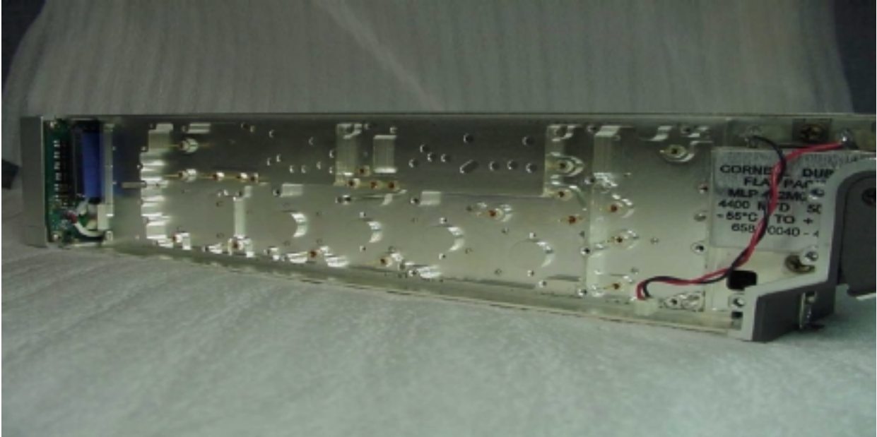
The chassis side of the Modulator/IF/Synthesizer, both the shield and the cover are removed.
