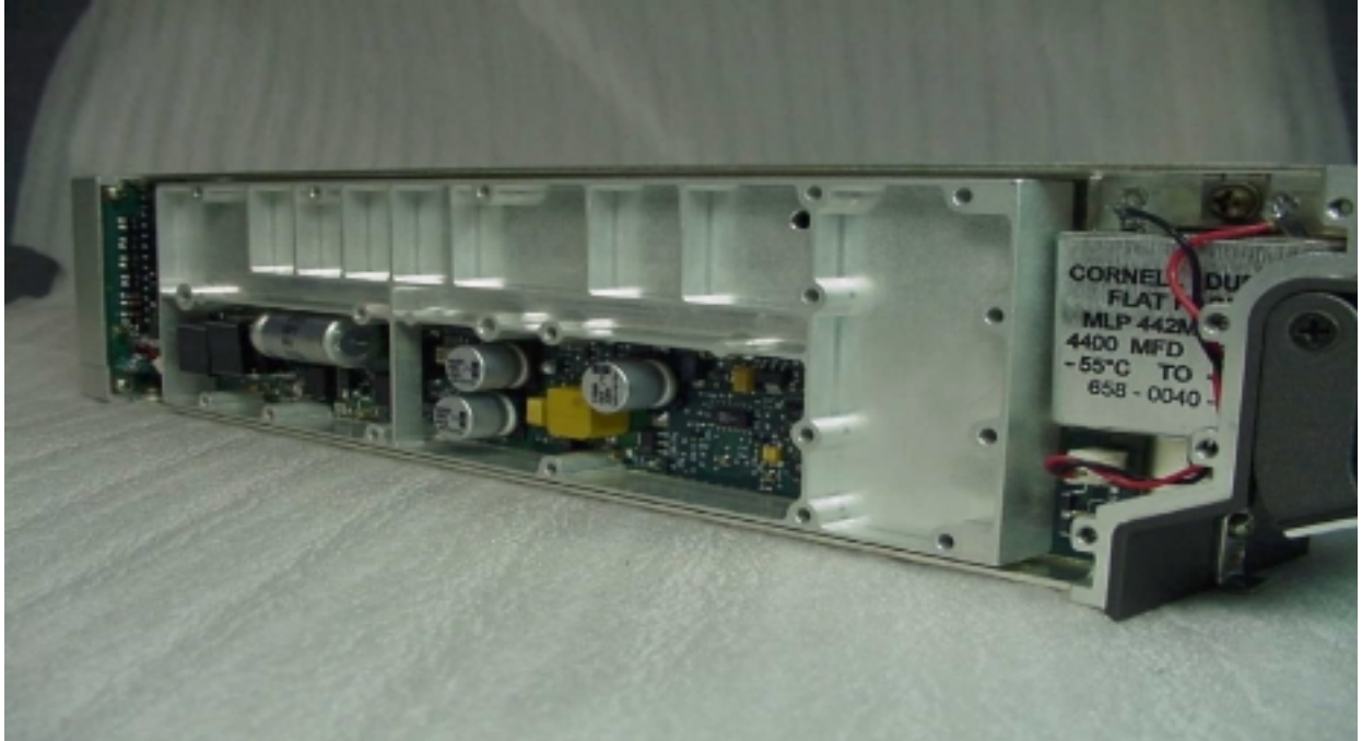
The DME4000 Modulator/IF/Synthesizer cover removed. The shield and the Modulator section of Modulator/IF/Synthesizer board are exposed. The IF and the Synthesizer section of the board are covered by the shield.
