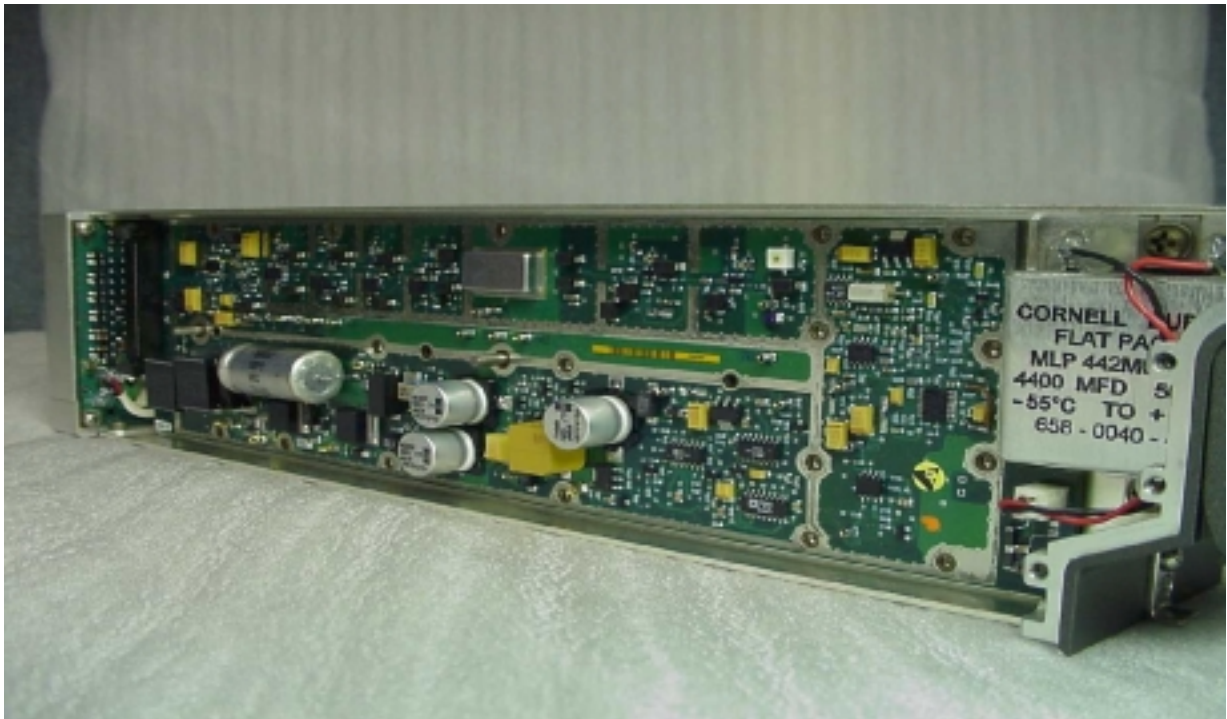
The DME4000 Modulator/IF/Synthesizer board with the shield removed.
