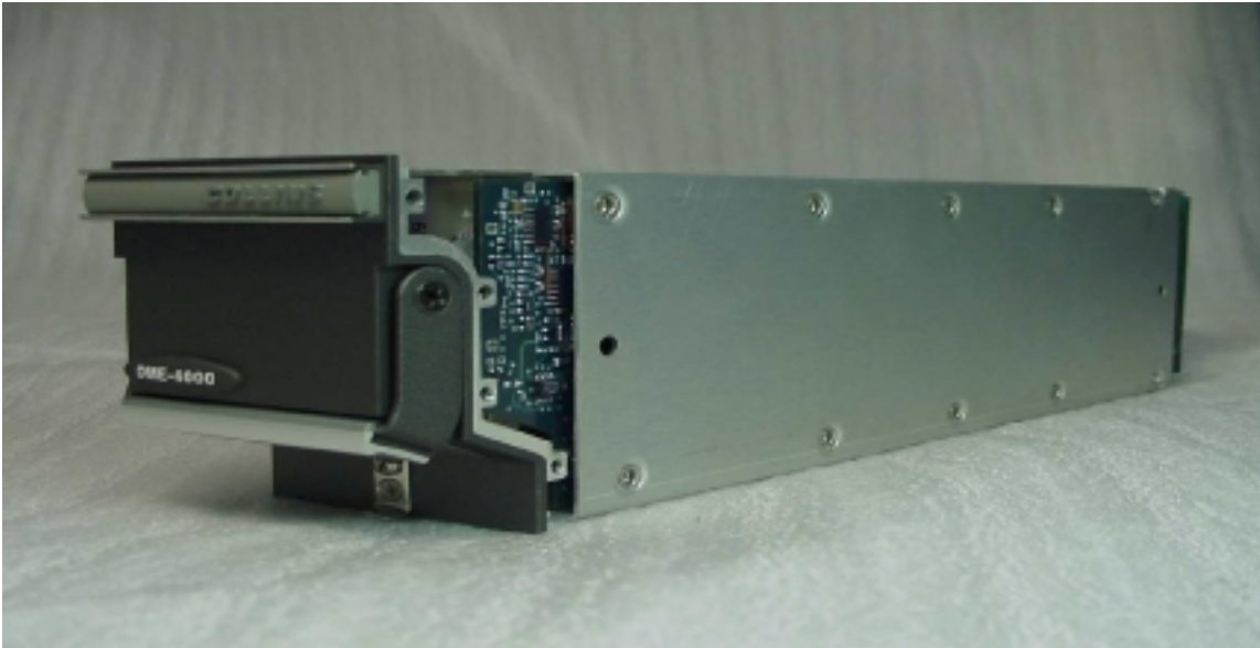
The DSP/Power Supply side of the DME-4000 with the unit cover removed.
