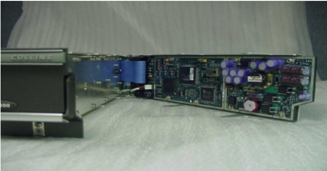
The DSP/Power Supply side is opened and the Radio Frequency Transmitter and Receiver shield is exposed.
