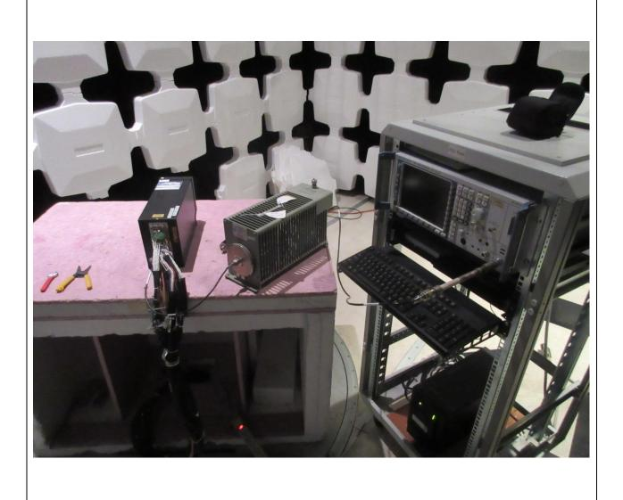
FIELD STRENGTH SPURIOUS EMISSIONS TEST SETUP
