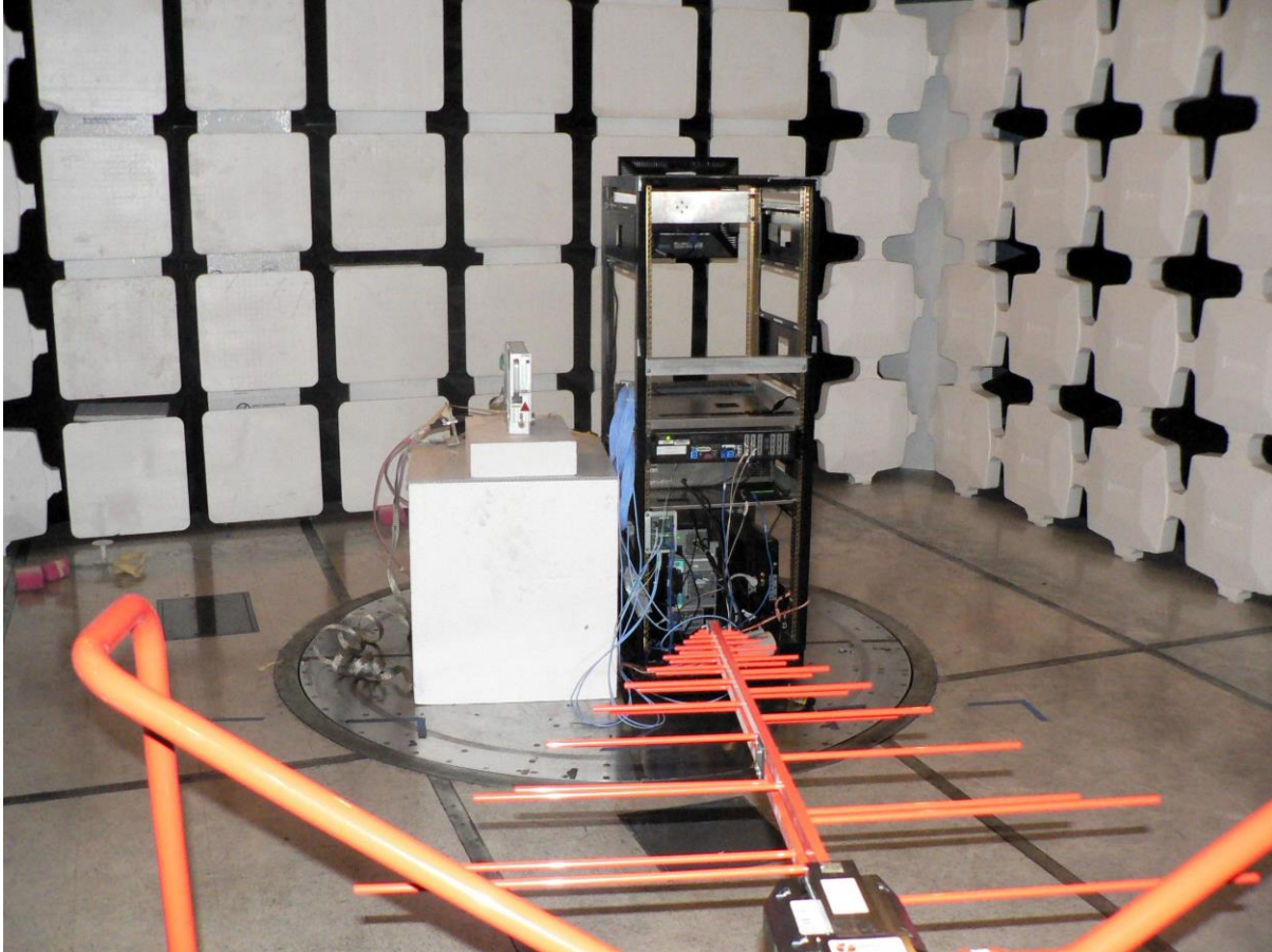
Radiated Emissions Setup – 30-1000 MHz Front
