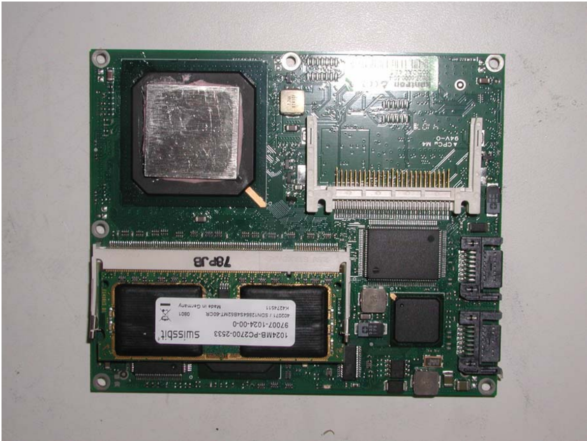
Figure I-7. UMTS-2100 ETLX Processor Board (CF memory removed) (top)
