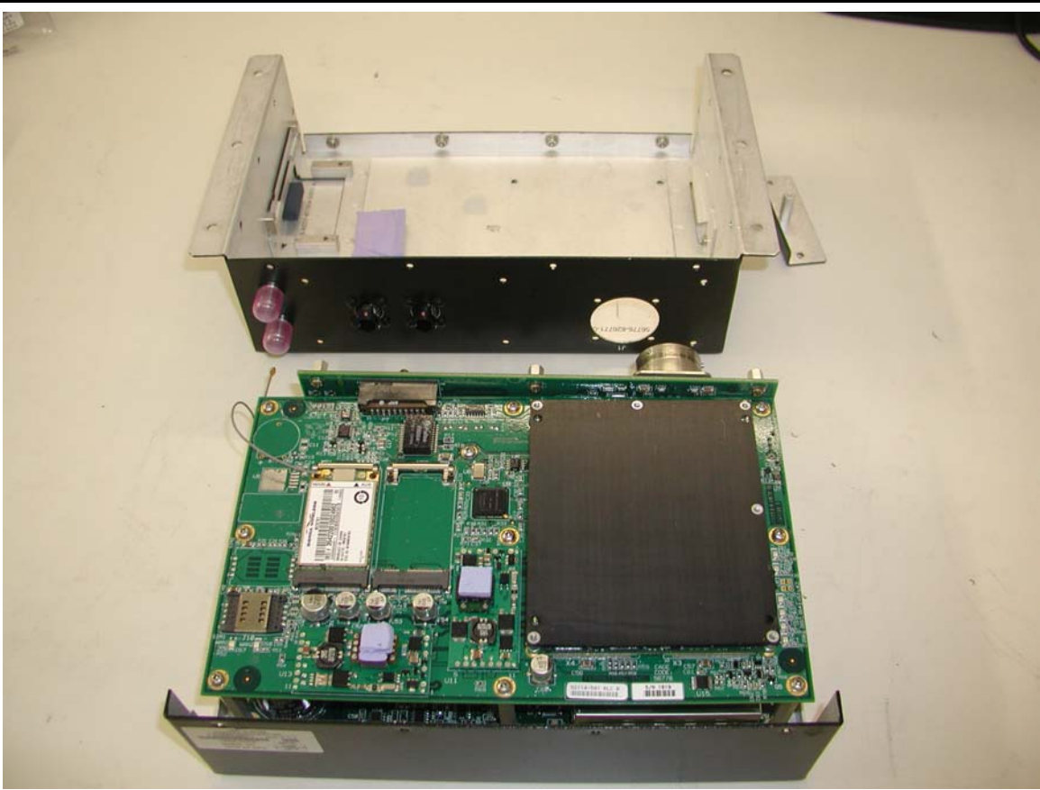
Figure I-1. UMTS-2100 with covers removed
