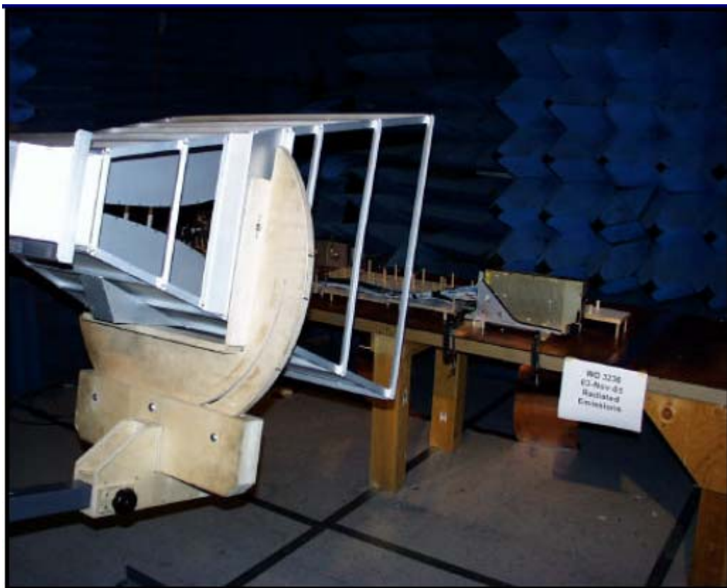
Figure 75. Radiated Emissions Test Setup-MPB
