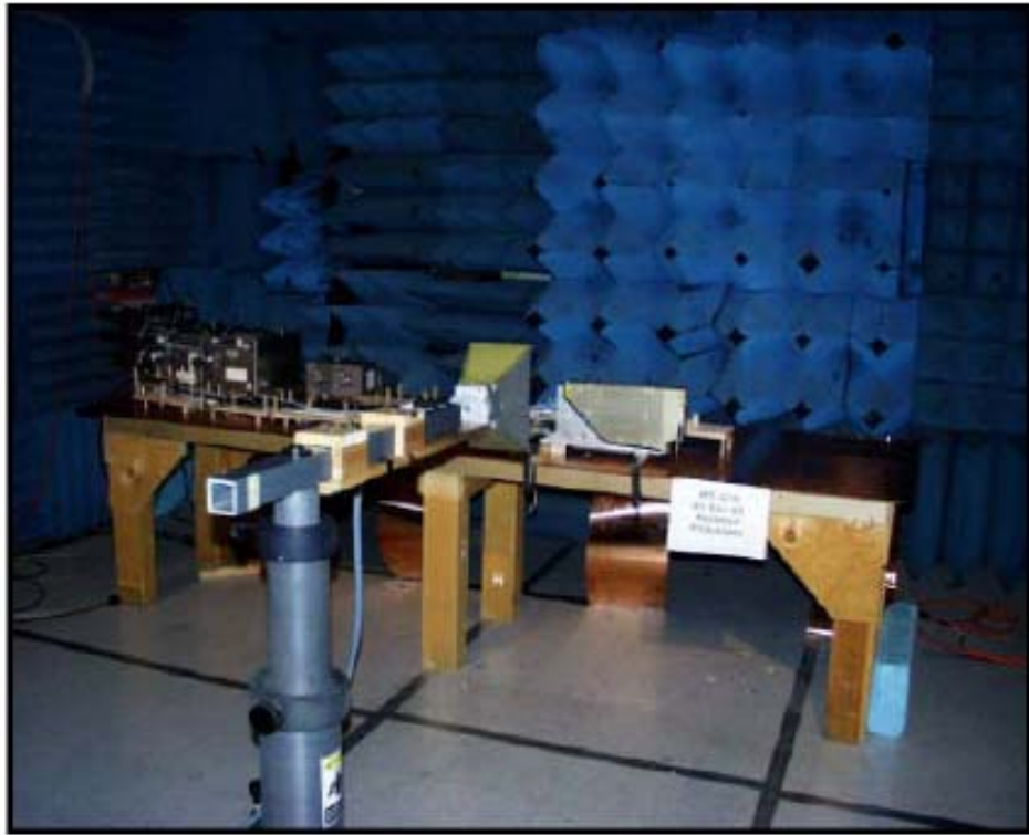
Figure 3 - Radiated Emissions Test Setup - MPB
