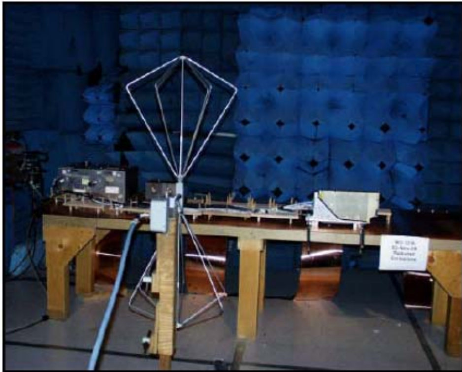
Figure 1 - Radiated Emissions Test Setup – MPB
