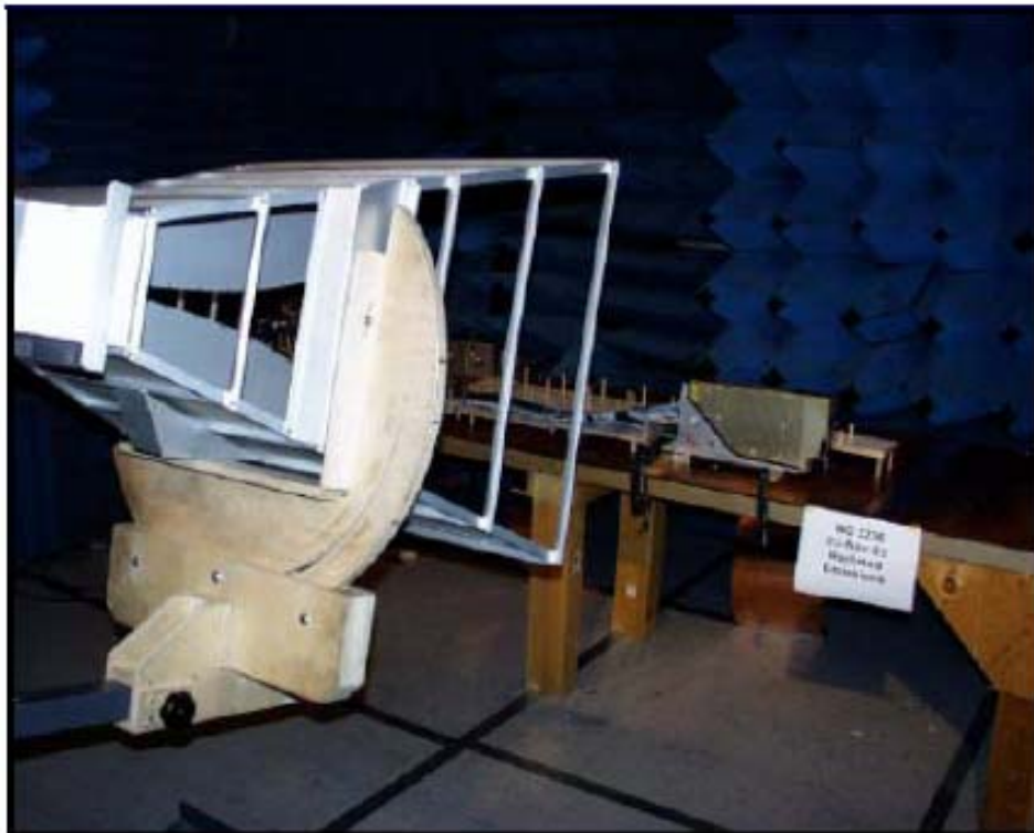
Figure 2 - Radiated Emissions Test Setup – MPB
