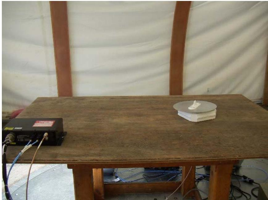
**RADIATED RF MEASUREMENT SETUP BELOW 1 GHZ WITH PATCH ANTENNA**
