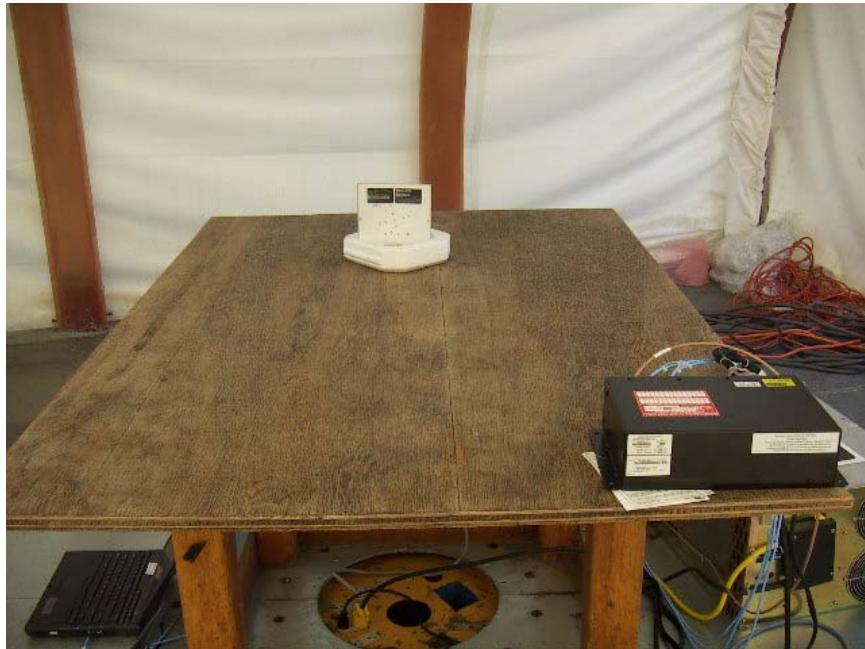
**RADIATED RF MEASUREMENT SETUP ABOVE 1 GHZ WITH AERODYNAMIC BLADE ANTENNA**
