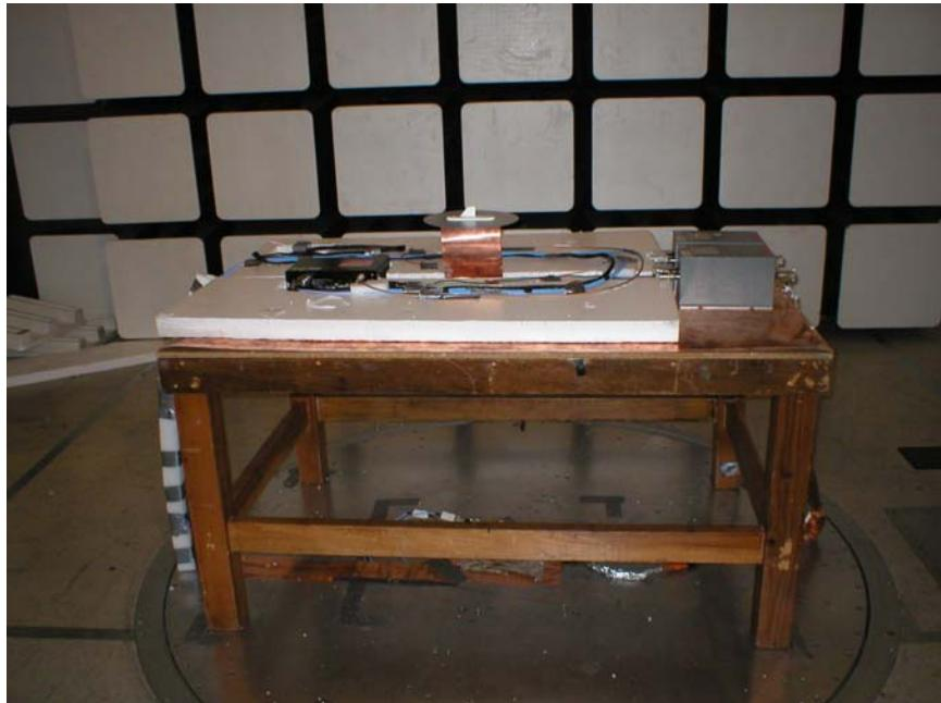
**RADIATED RF MEASUREMENT SETUP BELOW 1 GHZ – DETAILS OF CABLE ROUTING BETWEEN TABLE TOP GROUND PLANE AND CHAMBER GROUND PLANE**
