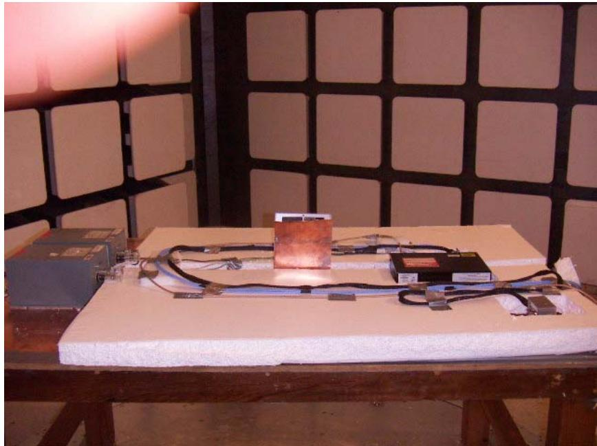
**RADIATED RF MEASUREMENT SETUP BELOW 1 GHZ WITH AERODYNAMIC BLADE ANTENNA**
