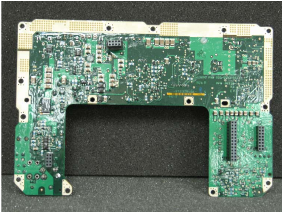
Figure I-11. Power Supply card (bottom)
