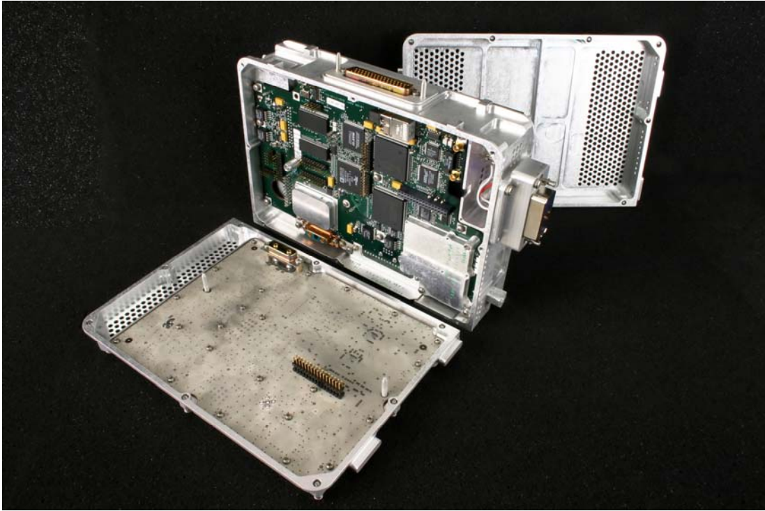
Figure I-1. RTM-2120 with covers removed
