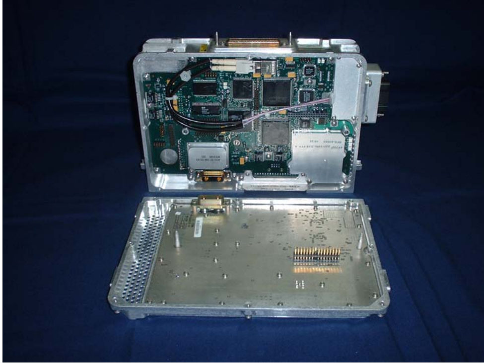
Figure I-3. RTM-2120 with DDS source removed
