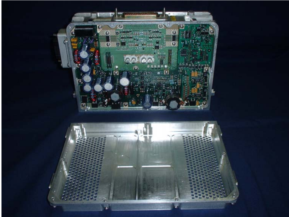
Figure I-2. RTM-2120 with power supply card exposed
