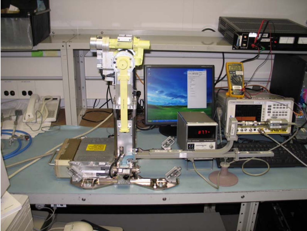
Figure G-1. Bench Test Setup – Occupied Bandwidth, Antenna Spurious, Power Line Stability
