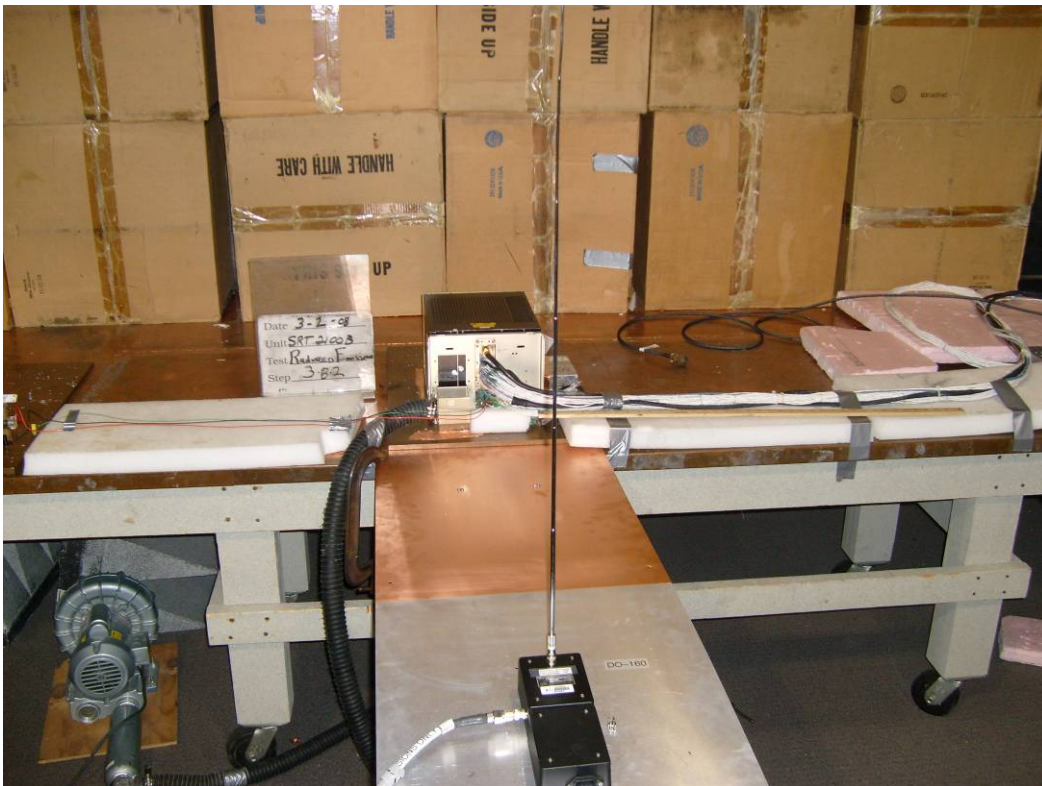
Figure 2 Field Strength of Spurious Radiation setup (2 MHz to 25 MHz)
