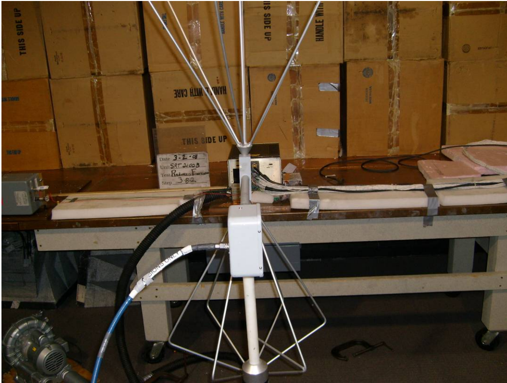
Figure 3 Field Strength of Spurious Radiation setup (25 MHz to 200 MHz)
