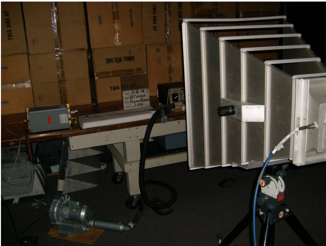
Figure 4 Field Strength of Spurious Radiation setup (200 MHz to 1 GHz)
