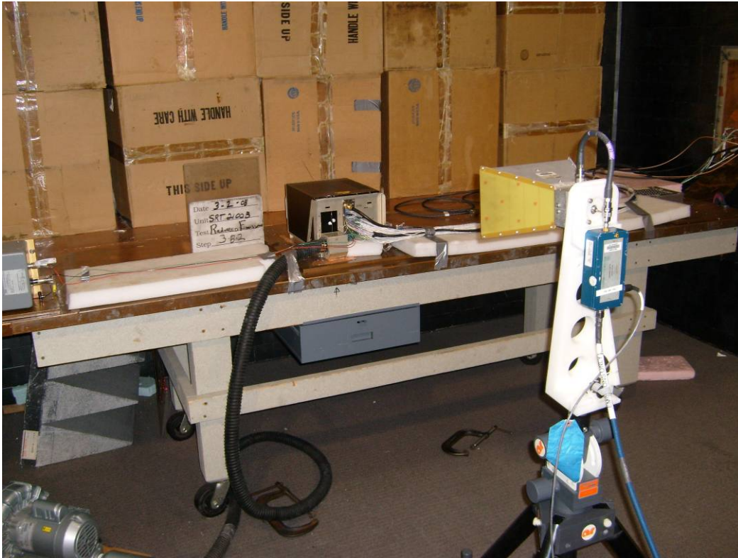
Figure 5 Field Strength of Spurious Radiation setup (1 GHz to 18 GHz)
