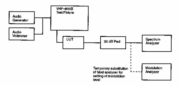
The test was repeated on 126.505 (8.33 kHz channel on 126.500 MHz) using modulating tones of 2500 Hz.
