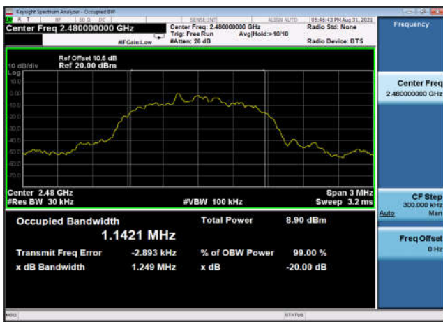
20dB Bandwidth: 8DPSK,2480MHz,3DH5
