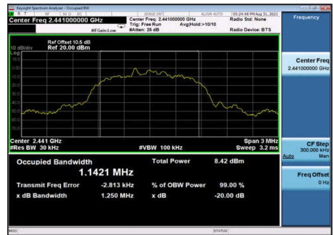
20dB Bandwidth: 8DPSK,2441MHz,3DH5
