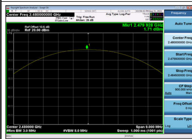
Output Power: DQPSK,2441MHz,2DH5
