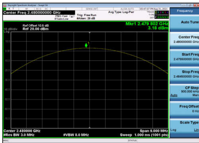
Output Power: 8DPSK,2480MHz,3DH5
