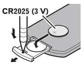
Insert the CR2025 (3 V) battery with the plus (+) and minus (-) poles orientated properly.
