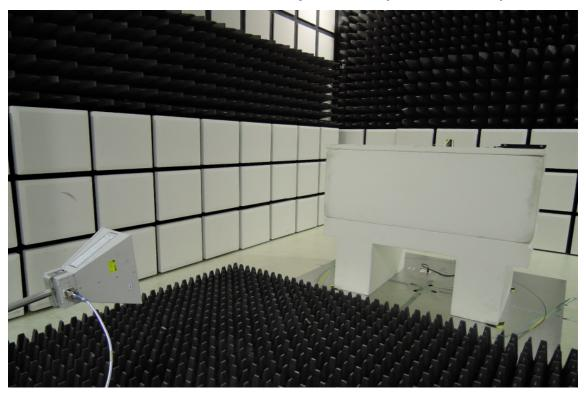
Radiated Emission Set up Photos (Front View)
