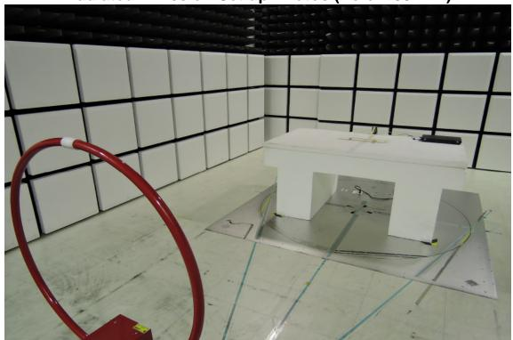
Radiated Emission Set up Photos (Below 1GHz)
