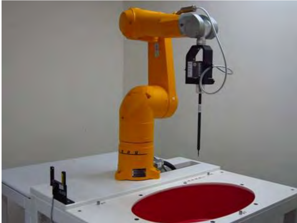
Fig.1 Photograph of the SAR measurement system
