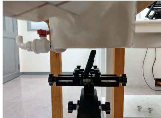
Fig.6 EUT Top Tilt side to flat phantom
