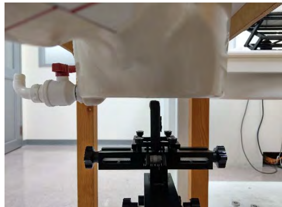
Fig.7 EUT Bottom side to flat phantom
