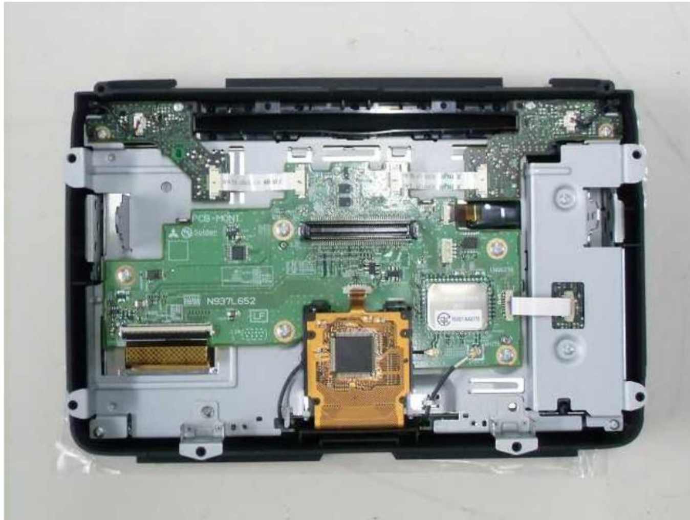
BT/WLAN Circuit Board on Grille Parts (Grille Parts Rear View)
