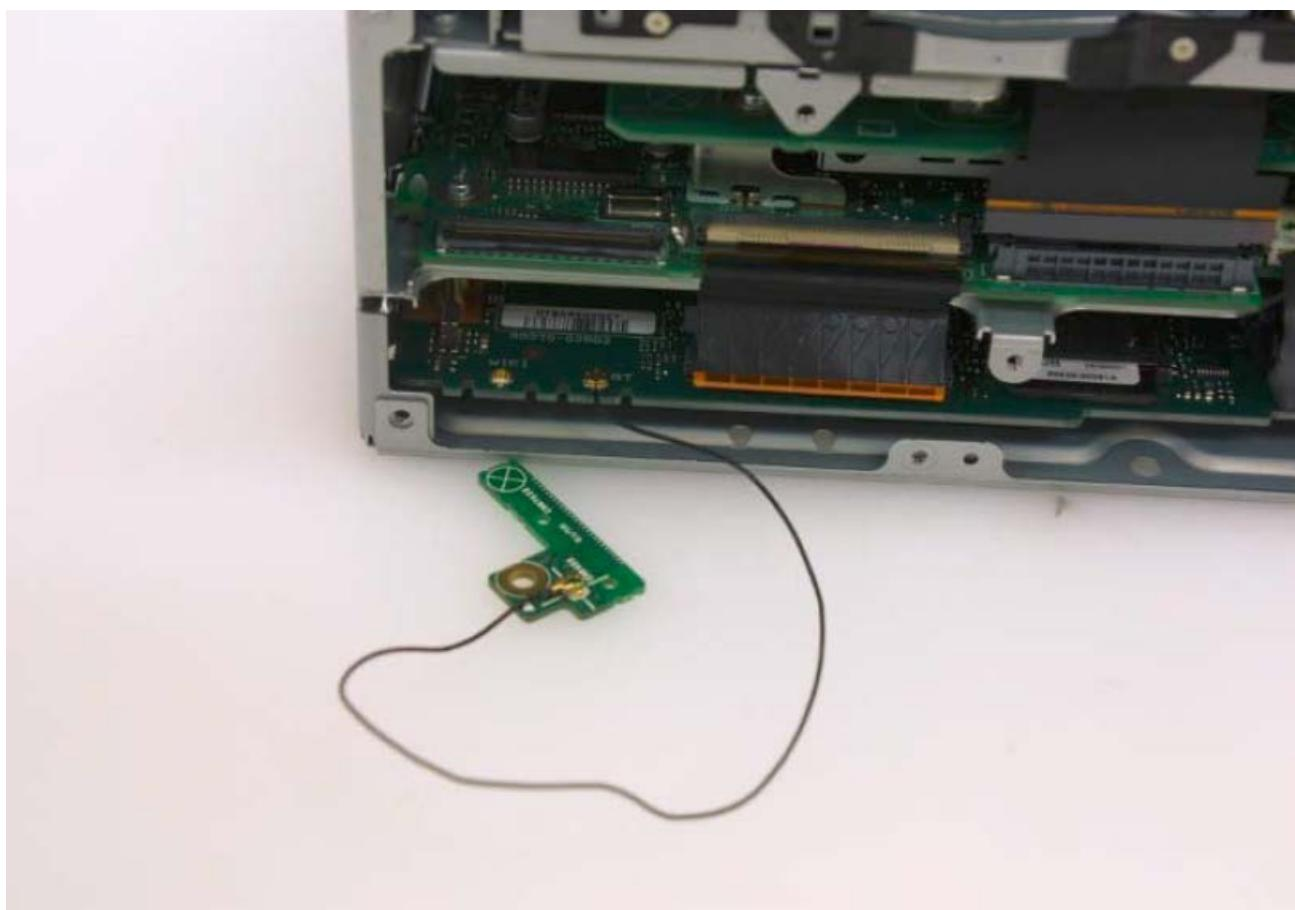
Internal Photo-antenna connection
