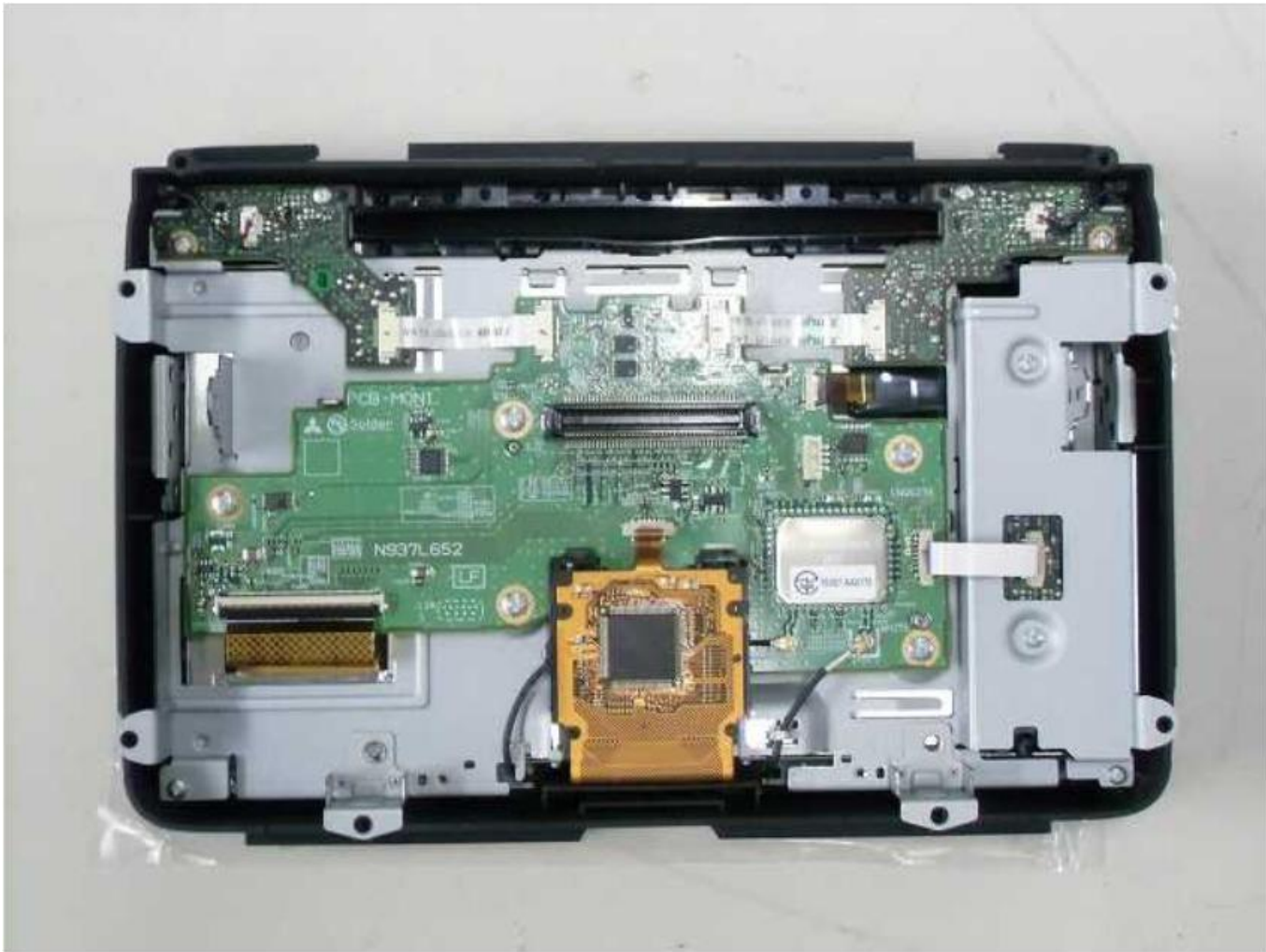
BT/WLAN Circuit Board on Grill Parts (Grill Parts Rear View)
