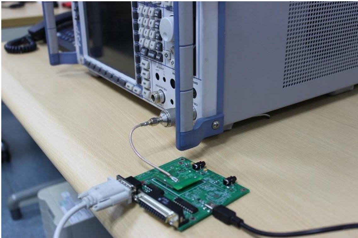
Photograph 1: Set-up for Conducted RF test at Antenna Port
