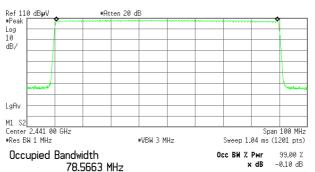
Transmit Freq Error -32.421 kHz x dB Bandwidth 18.941 MHz
