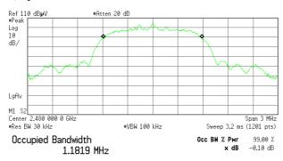
Transmit Freq Error -2.378 kHz x dB Bandwidth 11.106 kHz
