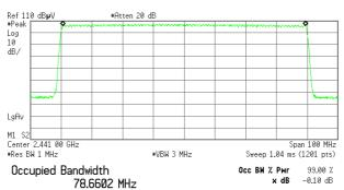
Transmit Freq Error -23.773 kHz x dB Bandwidth -6.015 kHz
