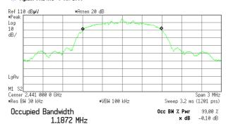
Transmit Freq Error -1.609 kHz x dB Bandwidth 8.843 kHz
