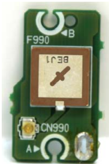
Front View of Antenna
