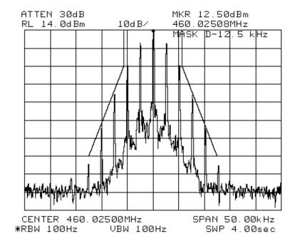
TYPE OF EXHIBIT: OCCUPIED BANDWIDTH- Digital 12.5 kHz CHANNELS
