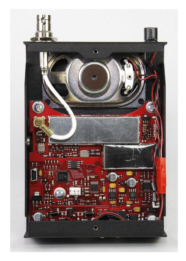
**EXHIBIT:** JBS-446D with case open to show printed circuit board installation
