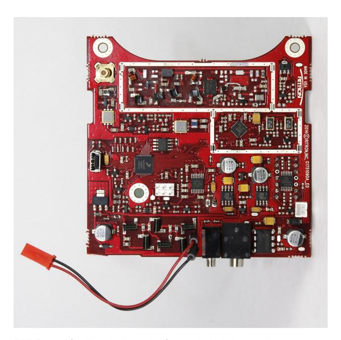
**EXHIBIT:** JBS-446D complete bottom side PCB assembly with shields removed
