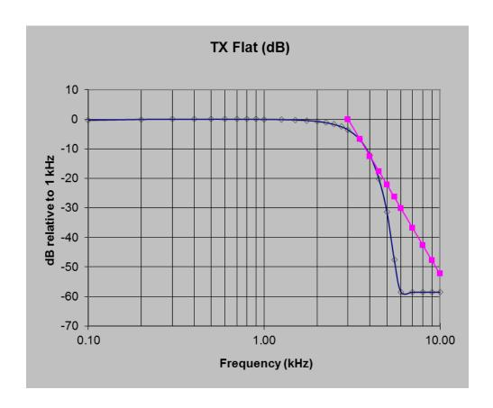
TYPE OF EXHIBIT: MODULATOR RESPONSE-12.5 kHz CHANNELS
