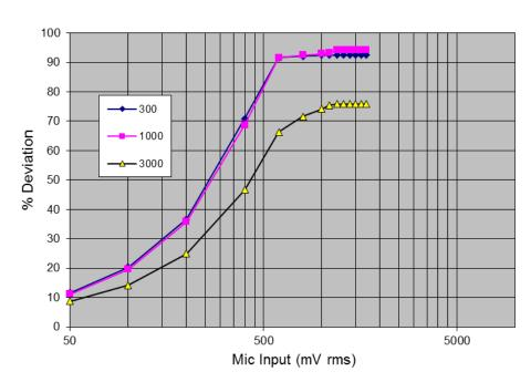
TYPE OF EXHIBIT: MODULATION LIMITING CURVES-12.5 kHz
