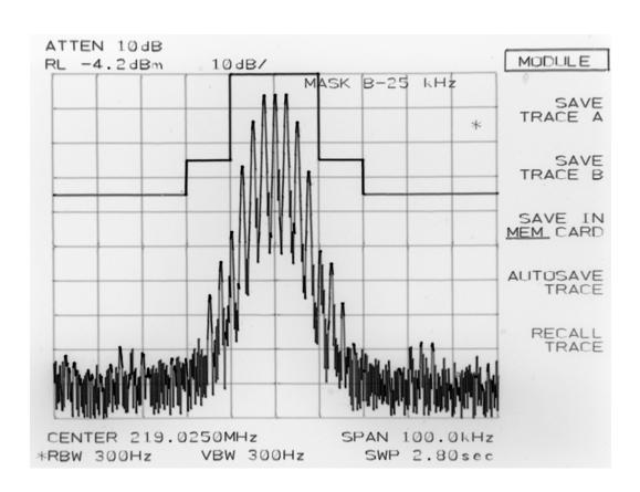
TYPE OF EXHIBIT: OCCUPIED BANDWIDTH-25 kHz CHANNELS
