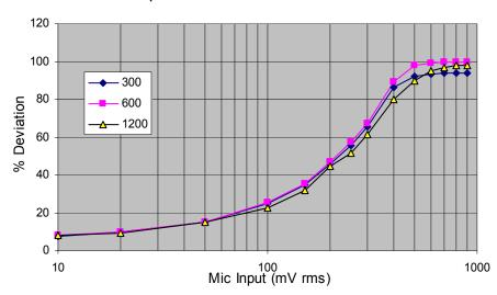
TYPE OF EXHIBIT: MODULATION LIMITING CURVES- 25 kHz
