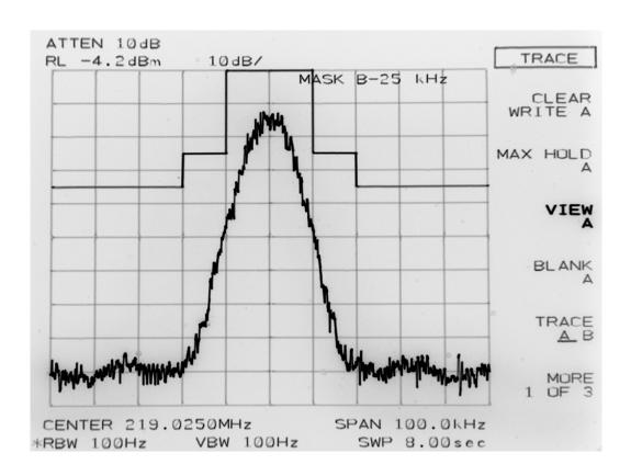
TYPE OF EXHIBIT: OCCUPIED BANDWIDTH-25 kHz CHANNELS
