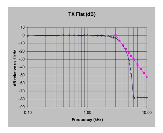
TYPE OF EXHIBIT: CLIPPER FILTER RESPONSE-6.25 kHz CHANNELS
