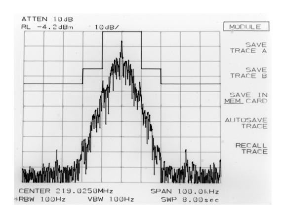
TYPE OF EXHIBIT: OCCUPIED BANDWIDTH-12.5 kHz CHANNELS
