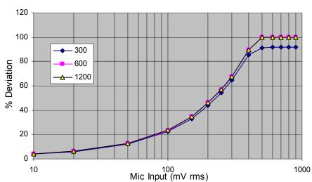
**TYPE OF EXHIBIT**: MODULATION LIMITING CURVES-12.5 kHz
