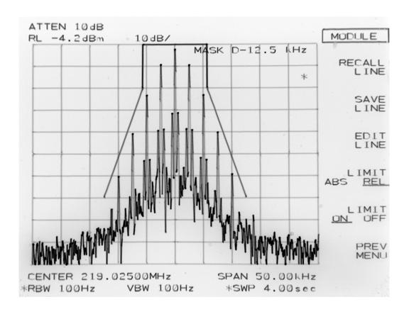
TYPE OF EXHIBIT: OCCUPIED BANDWIDTH-12.5 kHz CHANNELS
