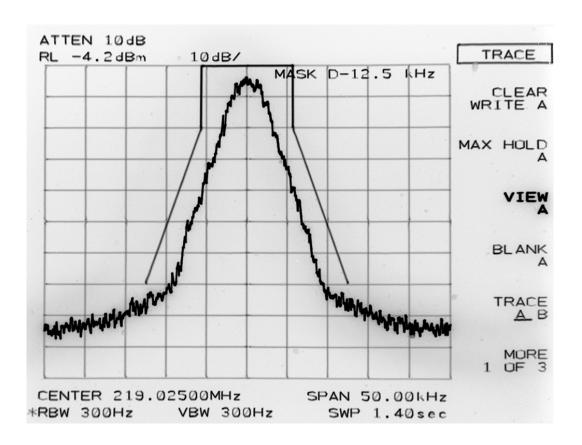
TYPE OF EXHIBIT: OCCUPIED BANDWIDTH-12.5 kHz CHANNELS
