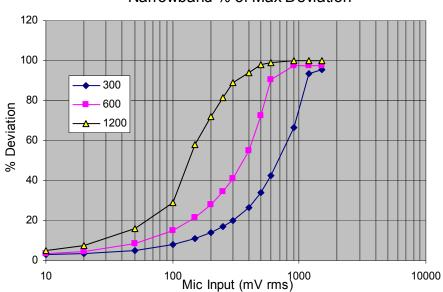
TYPE OF EXHIBIT: MODULATION LIMITING CURVES-6.25 kHz
