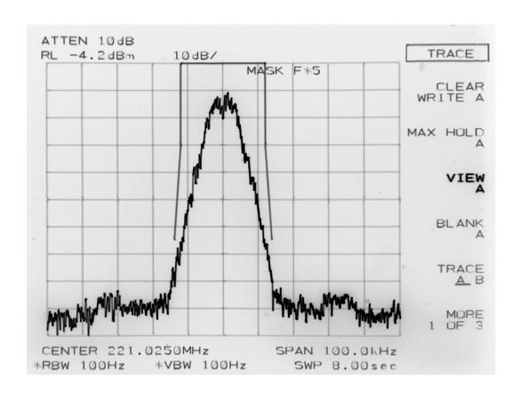
**TYPE OF EXHIBIT**: OCCUPIED BANDWIDTH- 5 kHz CHANNELS
