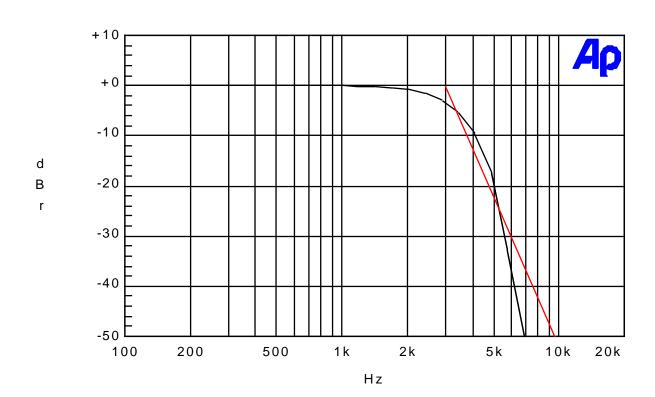
TYPE OF EXHIBIT: CLIPPER FILTER RESPONSE-6.25 kHz CHANNELS
