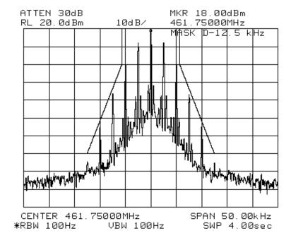
TYPE OF EXHIBIT: OCCUPIED BANDWIDTH-12.5 kHz CHANNELS
