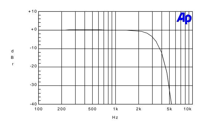
TYPE OF EXHIBIT: MODULATOR RESPONSE-12.5 kHz CHANNELS
