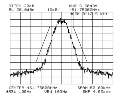
TYPE OF EXHIBIT: OCCUPIED BANDWIDTH-12.5 kHz CHANNELS
