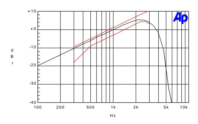
TYPE OF EXHIBIT: MODULATOR RESPONSE-6.25 kHz CHANNELS
