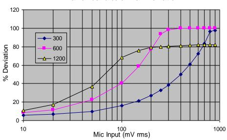
TYPE OF EXHIBIT: MODULATION LIMITING CURVES-6.25 kHz
