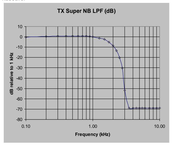
TYPE OF EXHIBIT: CLIPPER FILTER RESPONSE-12.5 kHz CHANNELS
