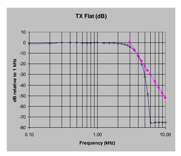
**TYPE OF EXHIBIT**: CLIPPER FILTER RESPONSE-6.25 kHz CHANNELS
