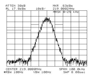
TYPE OF EXHIBIT: OCCUPIED BANDWIDTH-25 kHz CHANNELS
