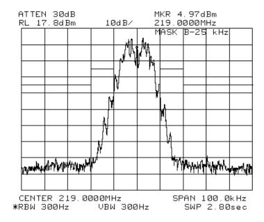
TYPE OF EXHIBIT: OCCUPIED BANDWIDTH-12.5 kHz CHANNELS
