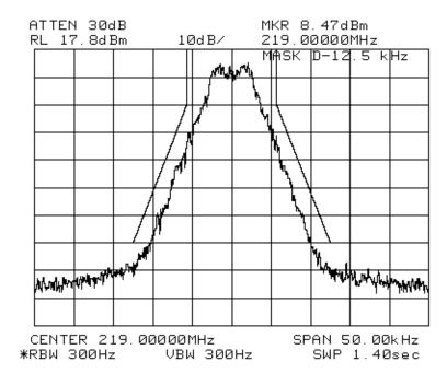
TYPE OF EXHIBIT: OCCUPIED BANDWIDTH-12.5 kHz CHANNELS
