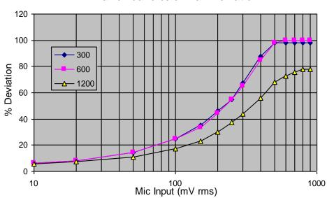
TYPE OF EXHIBIT: MODULATION LIMITING CURVES-12.5 kHz
