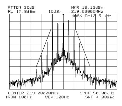
TYPE OF EXHIBIT: OCCUPIED BANDWIDTH-12.5 kHz CHANNELS
