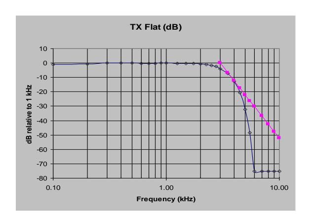
TYPE OF EXHIBIT: MODULATOR RESPONSE-12.5 kHz CHANNELS
