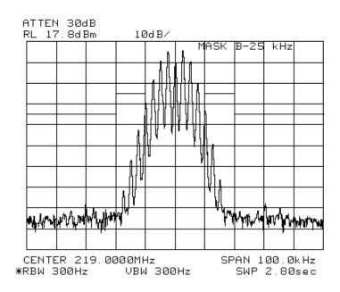
TYPE OF EXHIBIT: OCCUPIED BANDWIDTH-25 kHz CHANNELS
