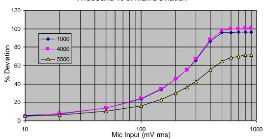
TYPE OF EXHIBIT: MODULATION LIMITING CURVES- 25 kHz
