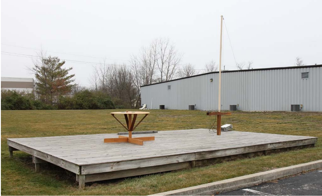
RQT-433-RCVR Radiated Spurious Emissions Test Setup Photos
