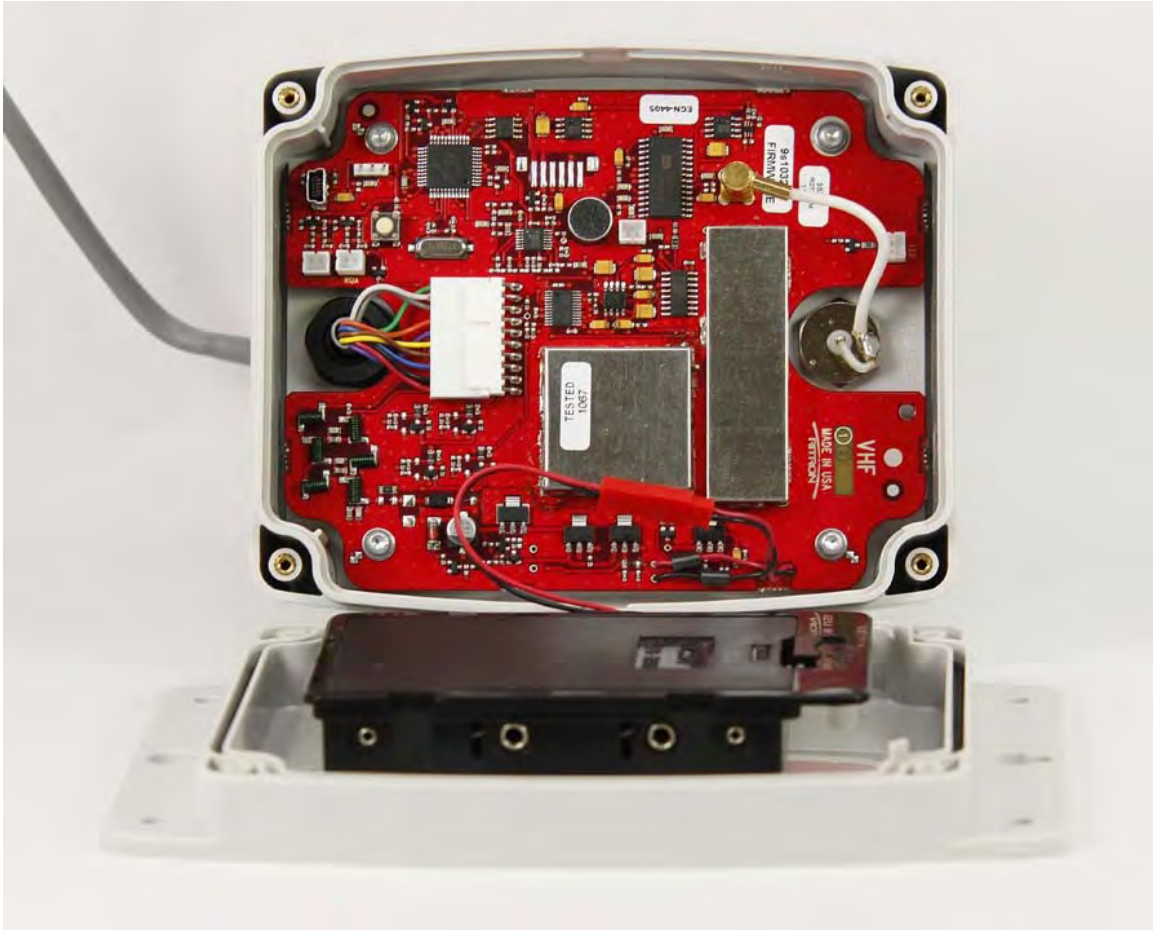
EXHIBIT: RQT-152M with case open to show printed circuit board installation FCC ID: AIERIT32-152M
