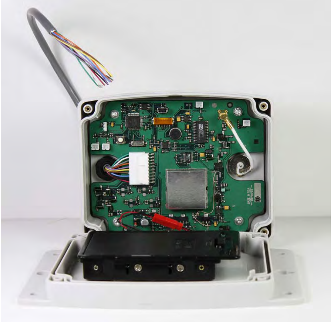
EXHIBIT: RQT-151M with case open to show printed circuit board installation FCC ID: AIERIT32-151M
