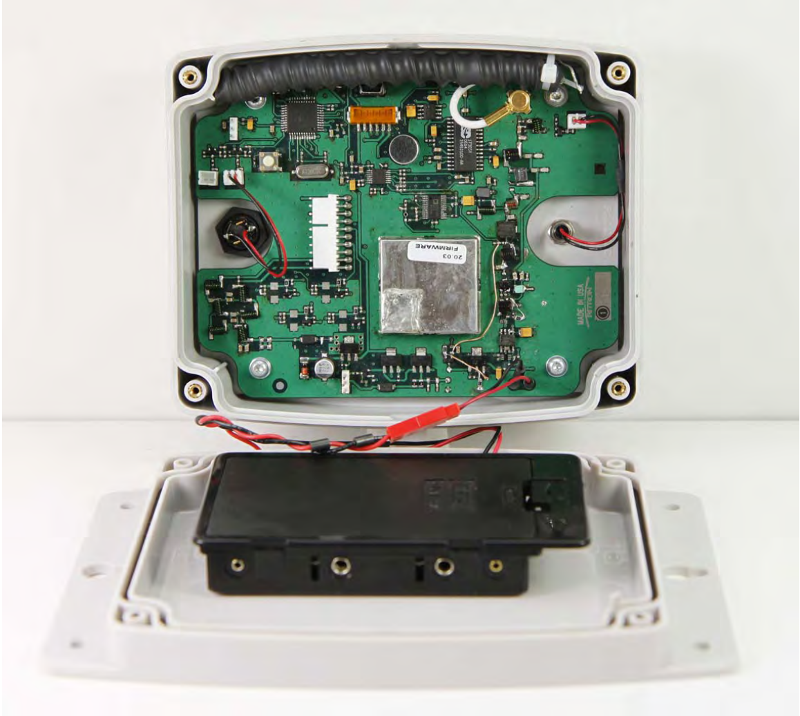
EXHIBIT: RQA-151M with case open to show printed circuit board installation FCC ID: AIERIT32-151M
