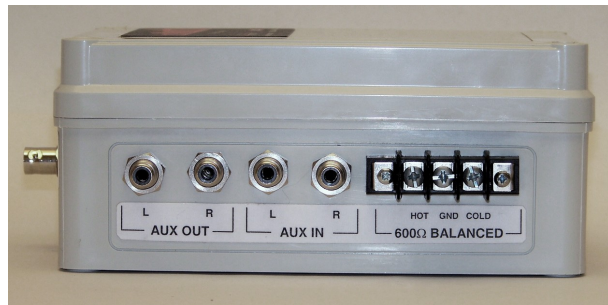
Side view showing high impedance unbalanced and 600Ω balanced audio outputs
