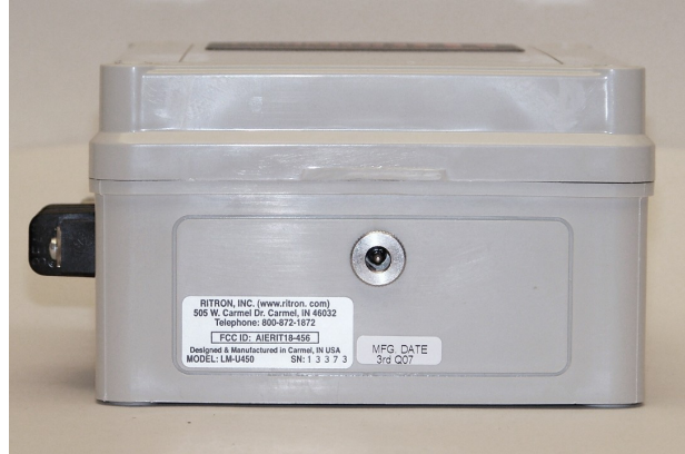
Bottom view showing DC power connector and location of FCC ID label
