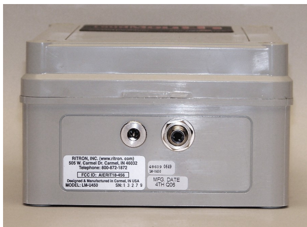
Bottom view showing DC power connector, horn speaker connector, and location of FCC/IC identification label
