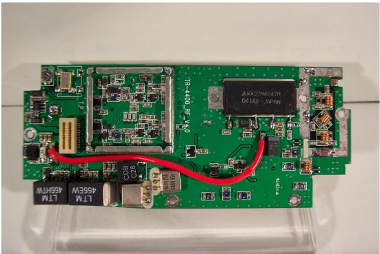
**EXHIBIT:** SPX-400 complete topside/bottomside RF PCB with shields removed
