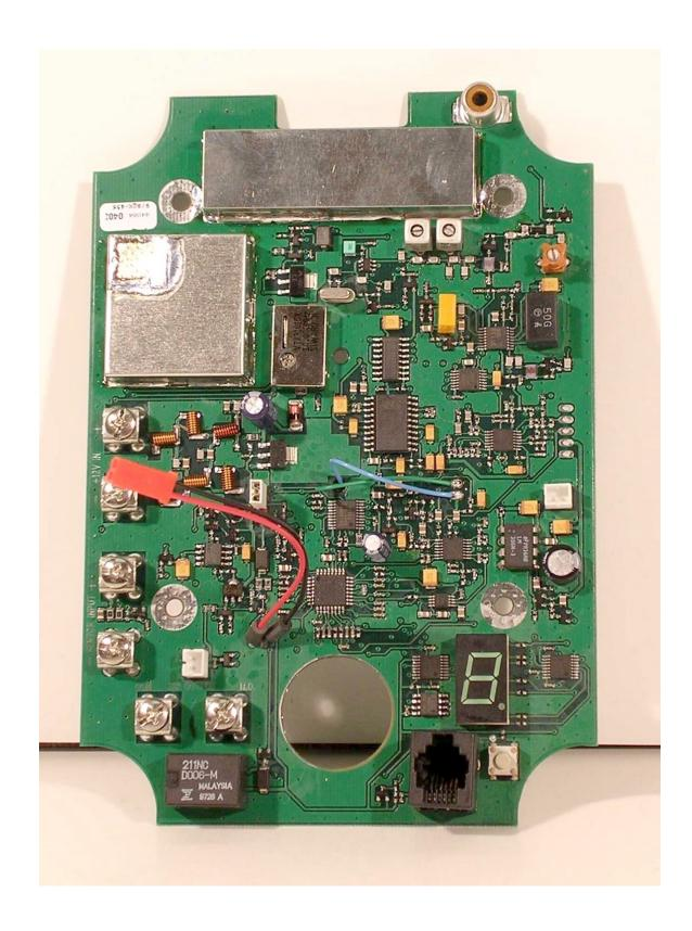
**EXHIBIT:** RQX-456 complete topside PCB assembly with shields installed
