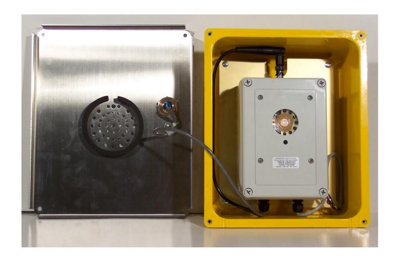
**EXHIBIT:** RQX-156-XT with front plate off to show installation of RQX-156 case assembly
