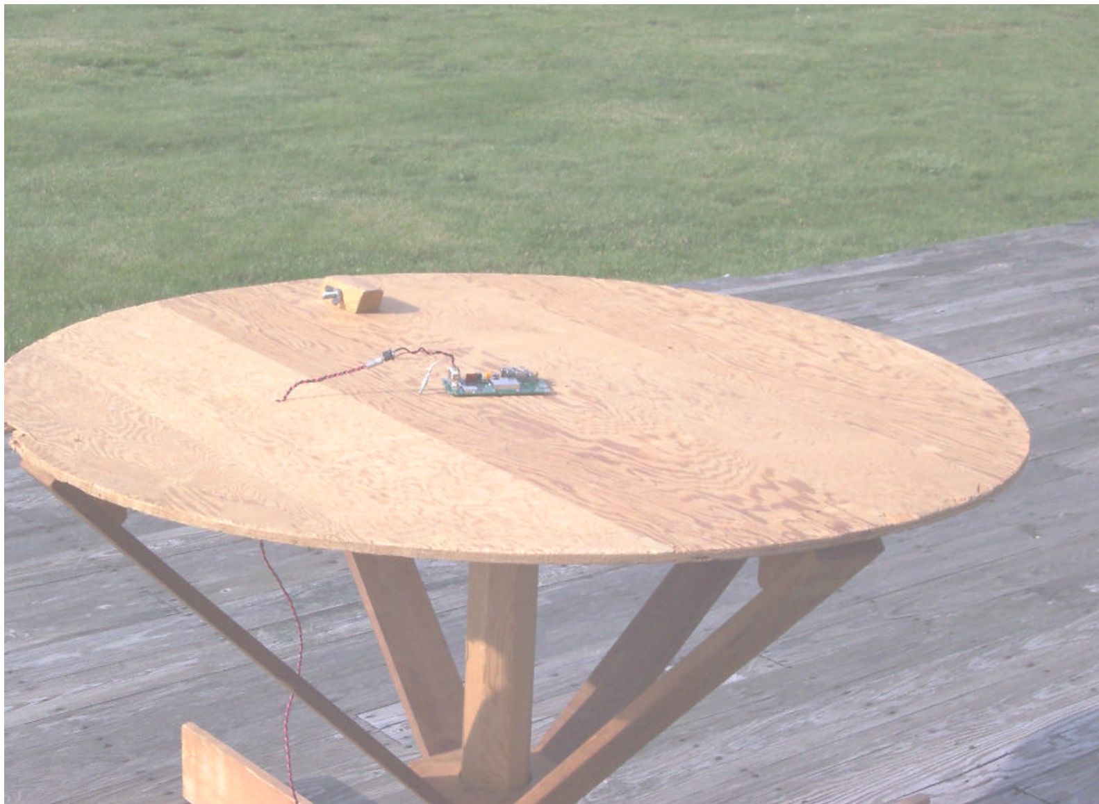
DR-442 on RITRON's 3 meter antenna range turntable
