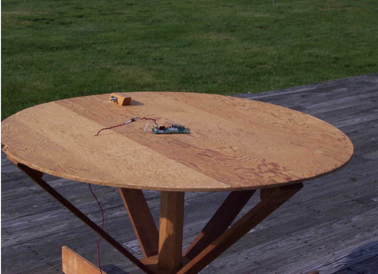
DR-142 on RITRON's 3 meter antenna range turntable
