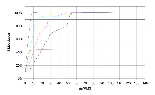
Channel Bandwidth: 25.0 kHz 100% Modulation: 5.0 kHz
