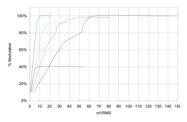
Channel Bandwidth: 12.5 kHz 100% Modulation: 2.5 kHz
