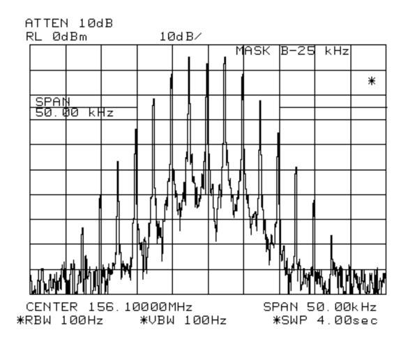
TYPE OF TEST: SPURIOUS EMISSIONS AT ANTENNA TERMINALS
