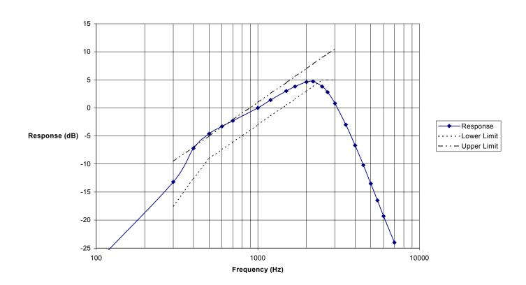
TYPE OF TEST: TRANSMIT AUDIO LOW-PASS FILTER RESPONSE
