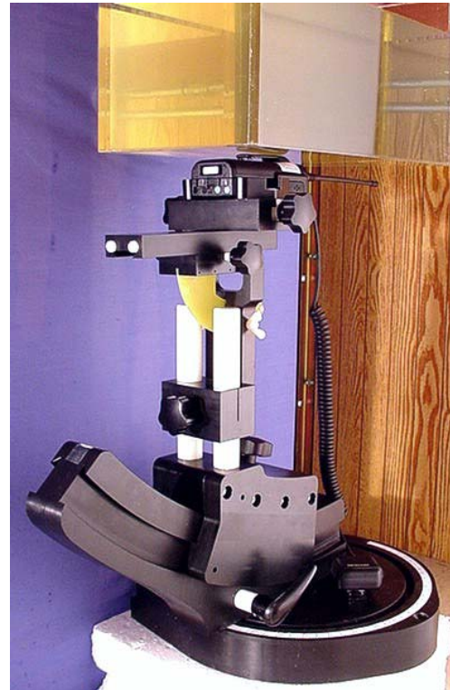
Body-worn SAR Test Setup
