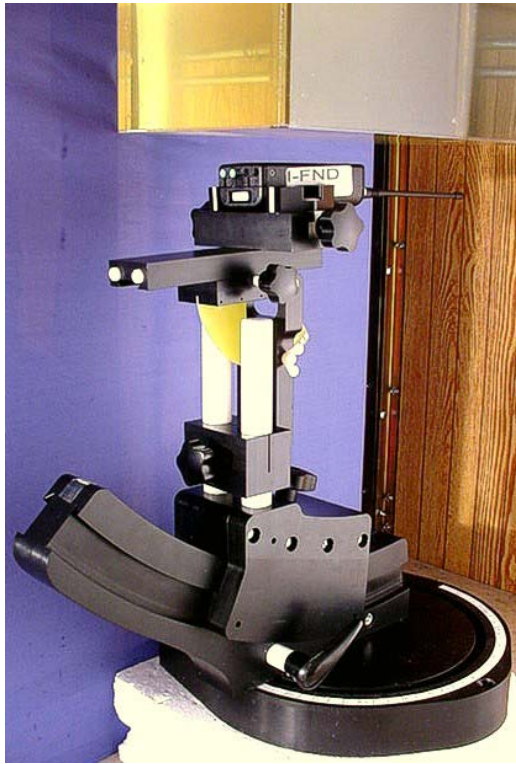
Face-held SAR Test Setup
