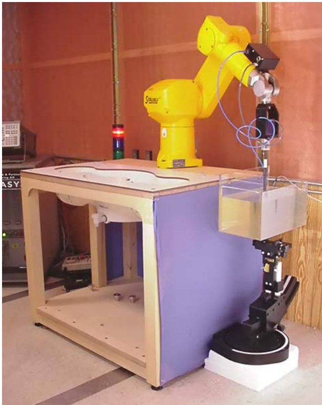
DASY3 SAR Measurement System with small planar phantom DASY3 SAR Measurement System with large planar phantom
