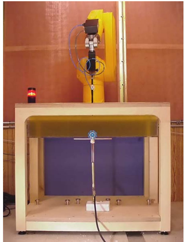
DASY3 SAR Measurement System with small planar phantom DASY3 SAR Measurement System with large planar phantom
