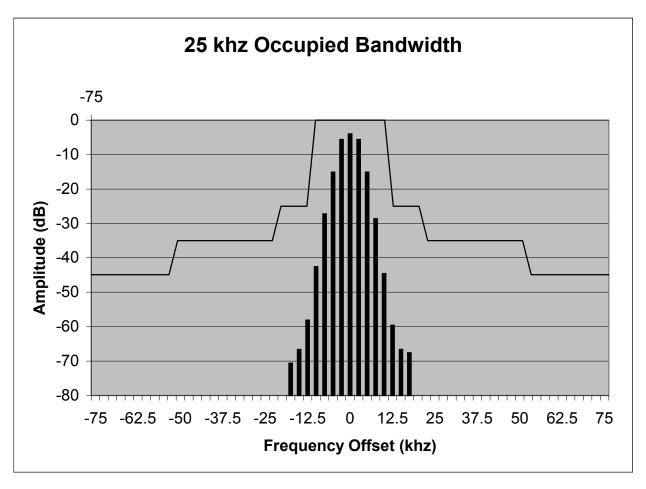
TYPE OF TEST: SPURIOUS EMISSIONS AT ANTENNA TERMINALS
