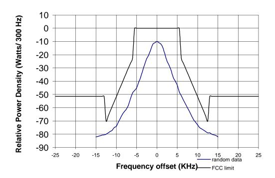
**TYPE OF TEST:** OCCUPIED BANDWIDTH for 9600 bps FSK DATA (11K2F1D)
