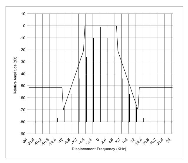
TYPE OF TEST: OCCUPIED BANDWIDTH for 1200 bps AFSK DATA (11K2F2D)
