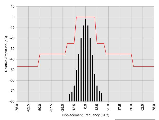
Channel Bandwidth: 25 KHz Power Output: 2.4 Watts 2500 Hz Sidebands
