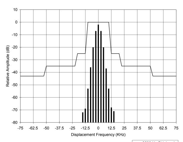
Channel Bandwidth: 25 KHz Power Output: 1.0 Watts 2500 Hz Sidebands
